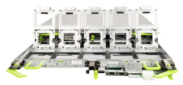
As with all OCP hardware the KNOX is designed for toolless maintenance. There are no caddies or screws – drives quickly snap into place.
